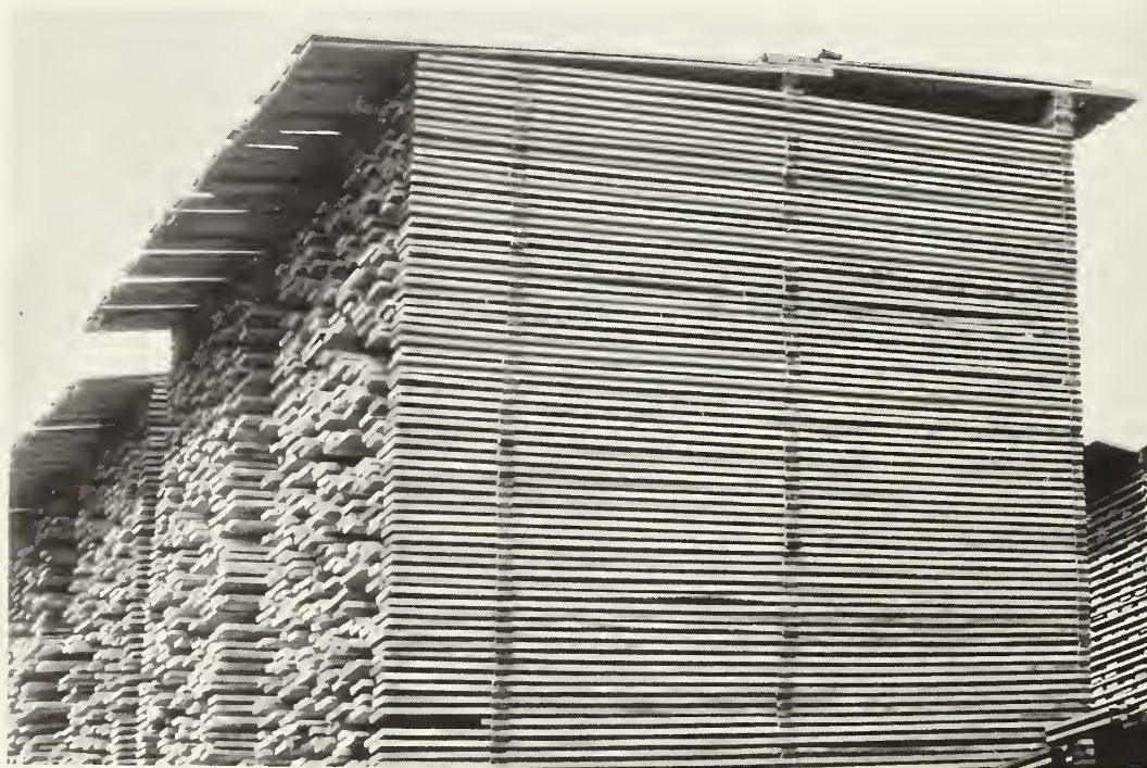
Figure 36. --Loose board roof on a sloped and pitched pile.
